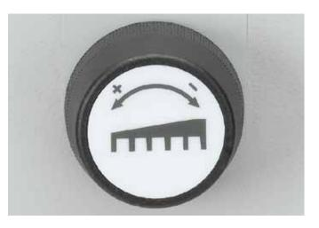
**ELECTRONIC HAND WHEEL** Electronic hand wheel for manual backgauge positioning with infinitely variable speed control (from very slow to very fast).
