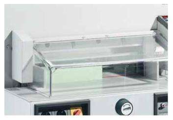
**SAFETY GUARD** The electronically secured front safety guard swings out of the way easily and allows safe and convenient cutting.
